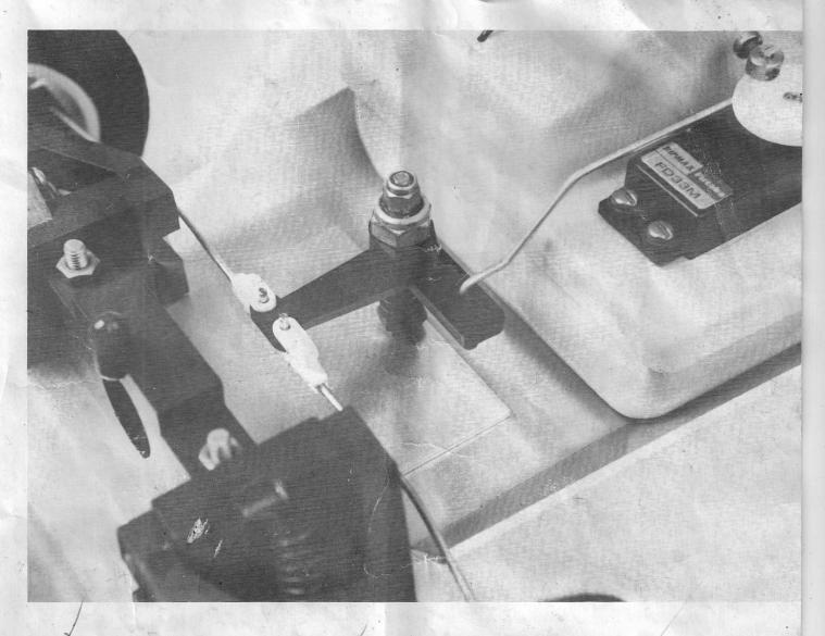
screws. Open up these holes in the lid to 3mm diameter. Mark out, drill, cut and file the aperture in the lid for the steering servo. Drill four holes 2.4mm diameter for self tap screws (93).
